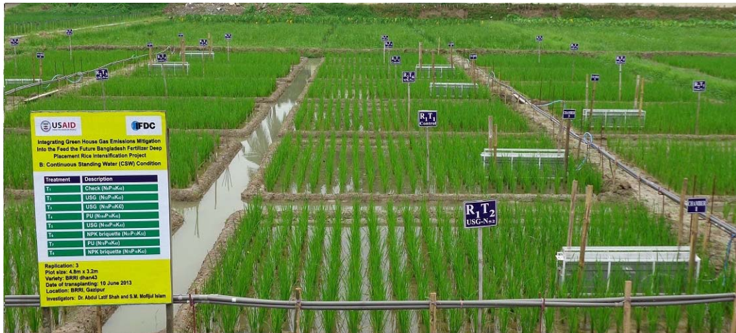
Photograph 1 Field view of GHG experiment at BRRI, Gazipur with gas chambers in the field
